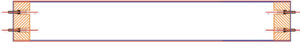
HIDDEN SPRING PIN CONNECTION DETAIL
